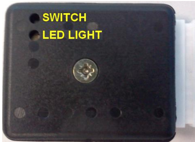
Figure 52 Adapter signaling led
